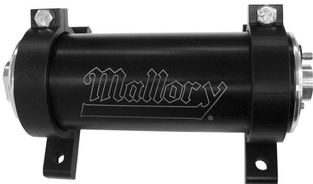
← When installing the pump, do not over tighten the nuts on the electrical posts. These need to be a **snug fit only**. Over tightening these connections can result in damaging internal connections and create a no run condition. This is considered damage at installation and not warrantied.
