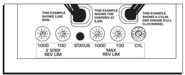
Figure 2 Rev Limiter sample setting.
