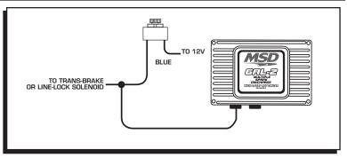
Figure 3 Wiring the 2-Step Rev Limit.
