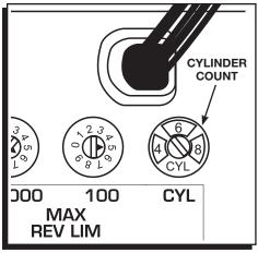
Figure 1 Programming the Number of Cylinders.
