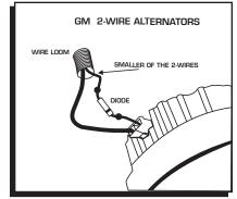
Figure 7 Installing the Diode to a 1973-1983 GM Vehicle.
