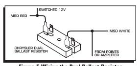
Figure 5 Wiring the Dual Ballast Resistor.
