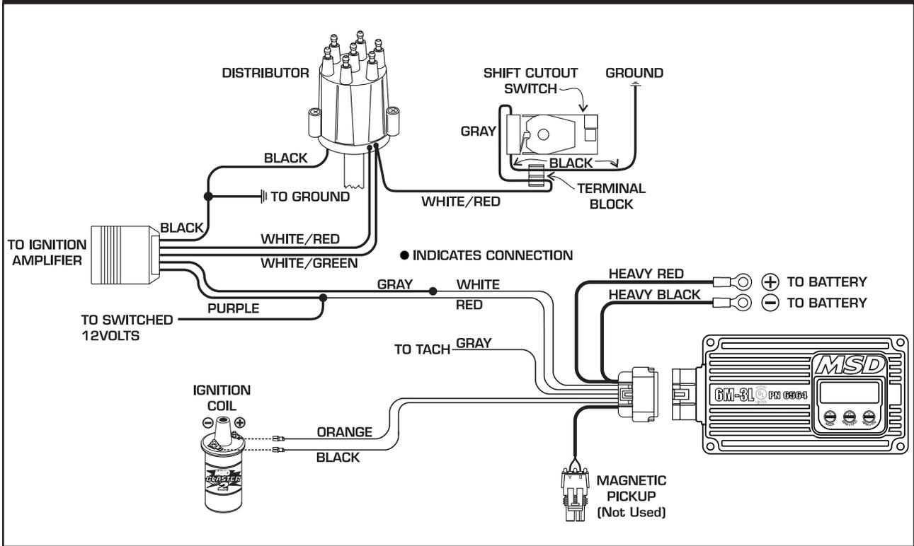
**MSD SYSTEMS Digital 6M-3L Marine Ignition to GM Dual Connector Coil**
