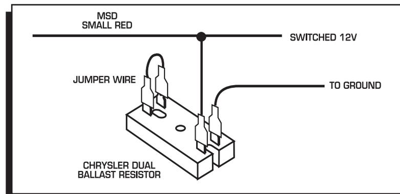
Figure 6 Wiring the Dual Ballast Resistor for Run-On.
