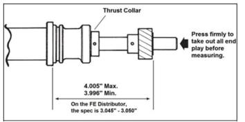
Figure 23 Gear Installation Specifications
