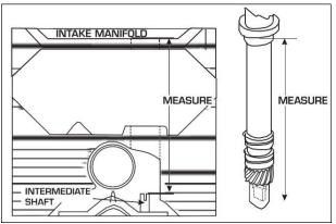
Figure 24 – Measuring Oil Pump Shaft Overlap
