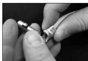
6. Slightly bend the terminal tabs over with pliers. DO NOT OVER CRIMP. This step is intended to secure the wire and terminal together and prepare for final crimping.
