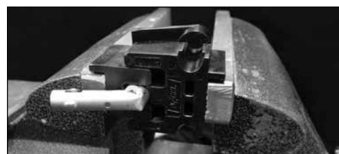
9. Once the terminal is closed around the wire, stop applying pressure. DO NOT OVER CRIMP. It is possible to over crimp the terminal and tear the silicone wire sleeve.
