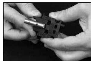
8. Assemble the crimp tool and place the alignment tabs into the jaws of the vise. Slowly close the vise, paying attention to the alignment of the terminal.
