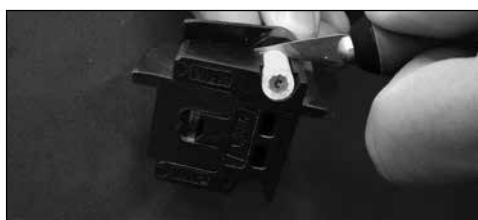
5. Fold the core over the wire. Insert the wire into the terminal and position the wire's silicone insulation 1/8" past the terminal's crimping tabs.
