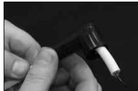
3. Utilizing the 7mm or 8mm holes on the ACCEL Wire Crimper, slide the wire though the hole with the end flush.
