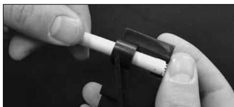
4. Holding a razor blade across the guide, rotate the wire and cut the circumference of the insulation. Be careful not to nick, cut or split the core. The exposed core should be 5/8".
