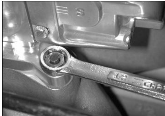
A socket or standard open-end wrench must be used to tighten the carburetor to the manifold.
