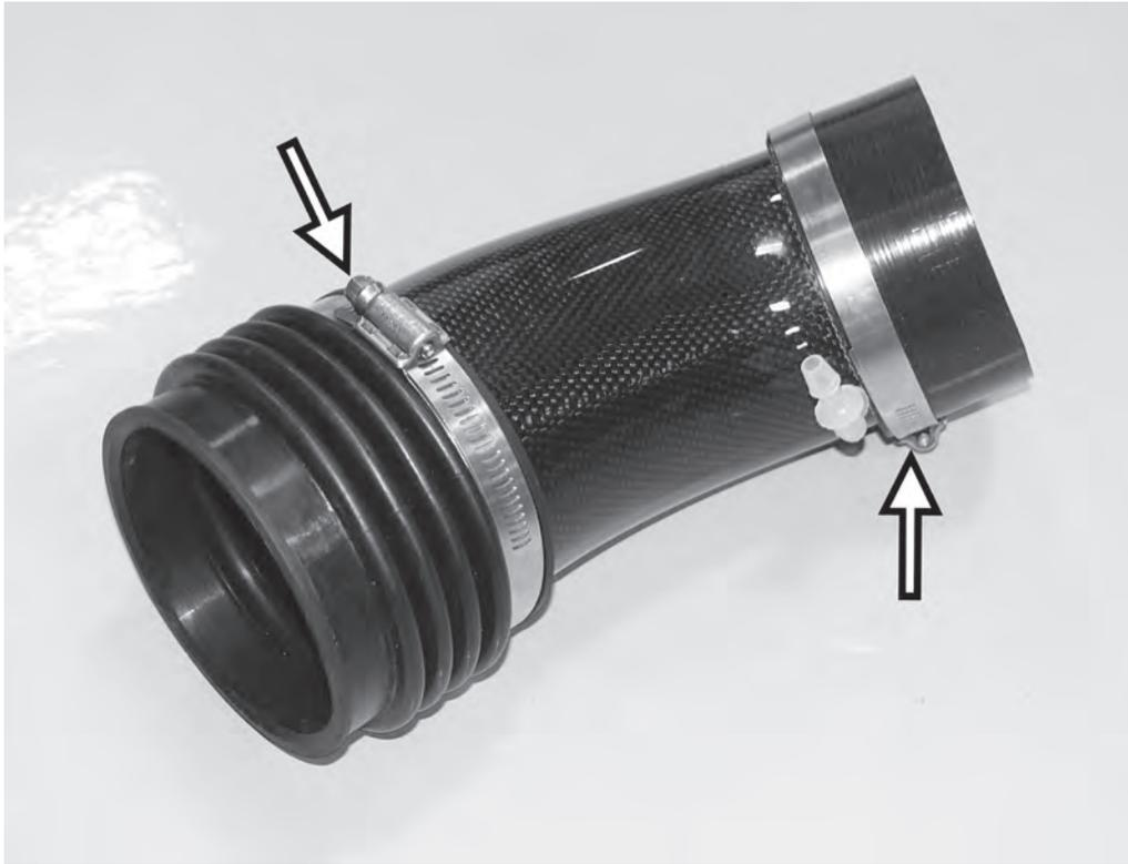
15) Install the silicone coupler on the end of the APR carbon fiber inlet tube with the supplied clamp. Install the accordion style coupler on the other end of the carbon fiber inlet tube and loosely secure with the supplied clamp.
