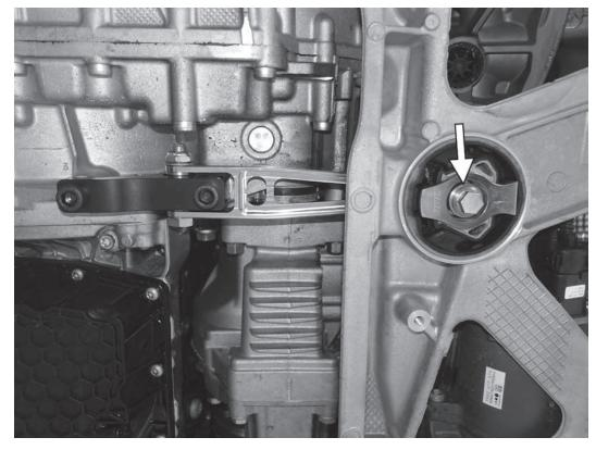
5) Reinstall either the 15mm bolt (if you have the APR subframe insert) or the 21mm stock bolt. It may be necessary to rock the engine/transmission assembly back to get the bolt started. If reusing the stock bolt, it is highly recommmended to replace this bolt. Torque the 15mm APR bolt to 100Nm (74lb-ft). Finally, torque the two 10mm allen bolts to 73Nm (54lb-ft).
