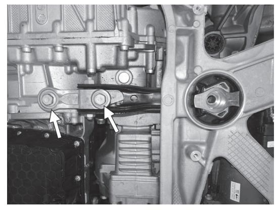
3) Remove the two 18mm bolts holding the dogbone mount to the transmission. Remove the stock dogbone mount and bracket from the car by sliding it forward from the slot in the front of the subframe.
