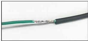
Soldered Connection w/ adhesive heat shrink
