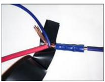
**Eletrical Taping Bare Wires**
