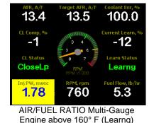
If any of these parameters are not showing a proper value, find out why before further driving the vehicle.
