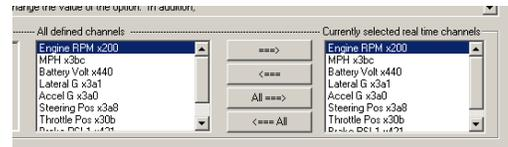
3. Select the desired channels to be viewed in real time from the All Defined Channels and place each channel (one at a time) in the Currently Selected Real Time Channel list by use of the > arrow, located between the two input areas. Channels maybe be removed from the Real Time list by using the < arrow. Complete this procedure for all desired channels.
