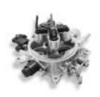
THROTTLE BODY INJECTION (TBI) — In TBI systems the throttle body assembly has two major functions: regulate the airflow, and house the fuel injectors and the fuel pressure regulator. The choices of throttle bodies range from single barrel/single
