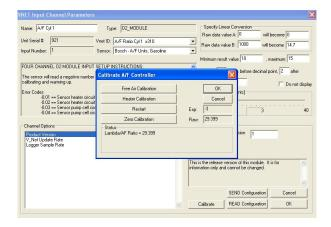
The status of the A/F channel will be displayed at the bottom of the 'Calibrate A/F Controller' dialog box that will appear. Before performing a calibration, make sure the sensor is not warming up or already performing a heater calibration. Also, make sure that there are no errors. If you have installed a new sensor in this channel first perform a zero calibration. Otherwise, perform a free air calibration. When you have finished click on the OK button to exit.
