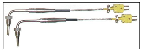
Attach the appropriate blue V-Net EGT module to each thermocouple using the yellow two prong connector. The V-Net modules will have EGT #1 or EGT #2 engraved on the back of the module. The #1 module should be attached to the front cylinder exhaust thermocouple, and #2 to the rear cylinder thermocouple.
