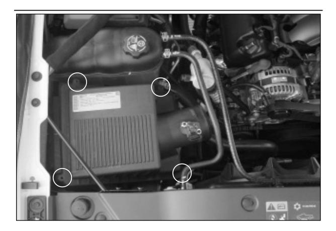
**STEP 7** - Remove the top portion of the stock intake housing by removing the 4 factory screws. Retain for later use.
