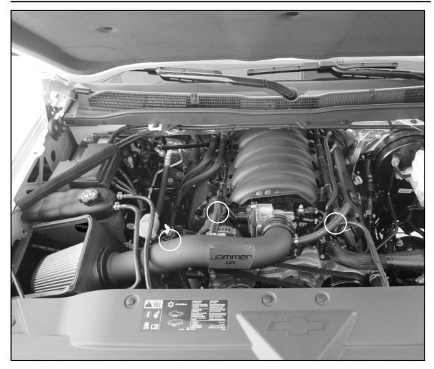
**STEP 16** - Install the crank case breathers onto both the passenger side and drivers side valve cover and attach it to the Jammer intake tube with the mini clamps and hose provided.
