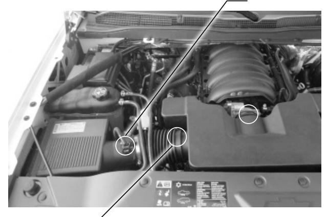
**STEP 2** - Loosen clamp from factrory air box housing and stock intake tube.
