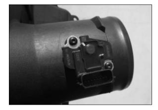
**STEP 9 -** Remove the MAF sensor from the stock housing.
