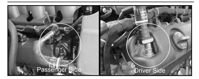
**STEP 5** - Disconnect the factory crank case breathers from the valve covers (as shown) on both sides of the engine.
