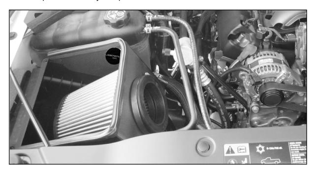
**STEP 14 -** Install the coupler onto the throttle body with provided clamps. Use the hump coupling for 5.3L models or the reducer coupling for 6.2L models.
