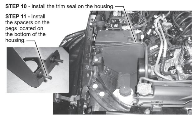
**STEP 12 -** Install the assembled housing into the vehicle as shown. Secure the housing using the OE bolt removed from Step 8.
