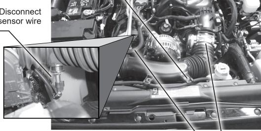
STEP 4 - Completely remove the small section of crankcase vent (CCV) hose. It should be pulled off of the air filter housing and the tube to the engine.
