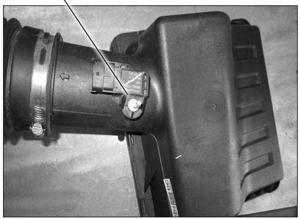
**STEP 14 -** Install the map sensor onto the Jammer intake tube using the hex head screw provided with a 10mm socket.  $\neg$
