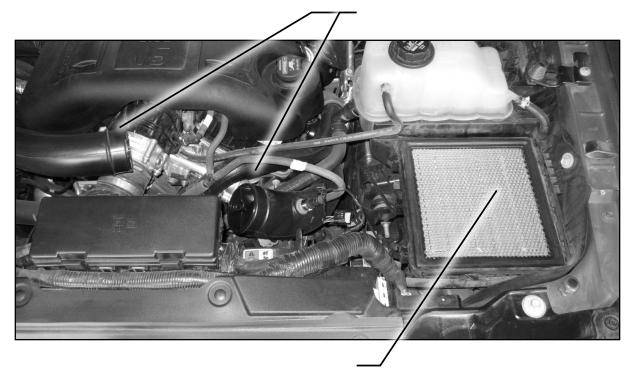
**STEP 5 -** Remove the stock filter from lower portion of the housing.
