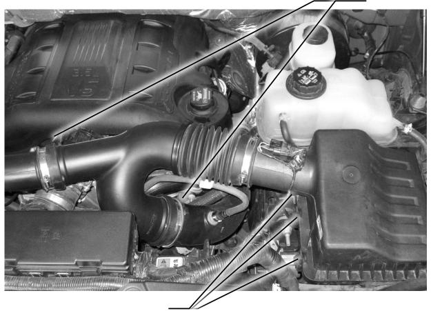
**STEP 3** - Unclip the 3 housing clips that secure the top portion of the stock intake housing.
