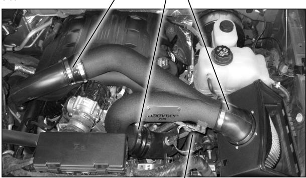
**STEP 16 -** Adjust the couplings and the tube for proper alignment and then tighten all clamps.
