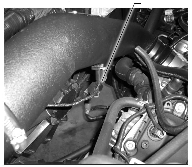
**STEP 17 -** Tighten the air filter clamp. Be sure not to over tighten or you can damage the filter base.
