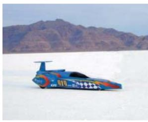
One of the most interesting examples of automotive technology featuring a motorcycle powerplant is the "Dreamliner." It is hand-built from 4130 chrome-alloy tubing and weighs in at 860 lbs. ready to run. The car measures 17' in length and is covered by aluminum in front and fiberglass in rear.
