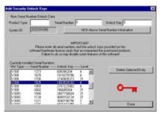
**Step 3:** The numbers you will need are in the Currently Installed Serial Numbers: window of the Add Security Unlock Keys box. They are in the columns titled HW Type, Serial Number, and Unlock Key. **Write these numbers down exactly as they appear**.
