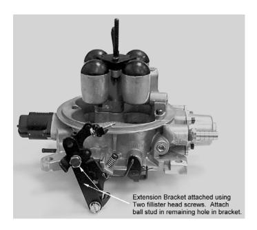
DANGER! STICKING THROTTLE MAY RESULT IN UNCONTROLLED ENGINE OR VEHICLE SPEED. THIS COULD CAUSE PROPERTY DAMAGE, PERSONAL INJURY, OR DEATH. A STICKING THROTTLE MAY BE CAUSED BY IMPROPERLY INSTALLED THROTTLE CABLES, LACK OF CLEARANCE FOR ANY OF THE THROTTLE LINKAGE, OR BY A BINDING THROTTLE LINKAGE. CHECK ALL THROTTLE CABLES FOR PROPER INSTALLATION AND ALIGNMENT AND ACTUATE THE THROTTLE TO CHECK FOR ANY POTENTIAL BINDING OR CLEARANCE PROBLEMS. REPAIR ANY PROBLEMS BEFORE CONTINUING.
