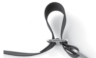
Figure 19 Place the Anchor as loose as possible to the 3-bar to reduce slipping. Lace the free end of the webbing thru both sides of the 3-bar.
