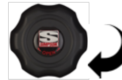
Figure 15 Rotate >30° to disengage lap belt tongues.
