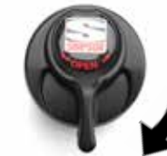
Figure 16 Rotate 20° to release lap belt tongues.
