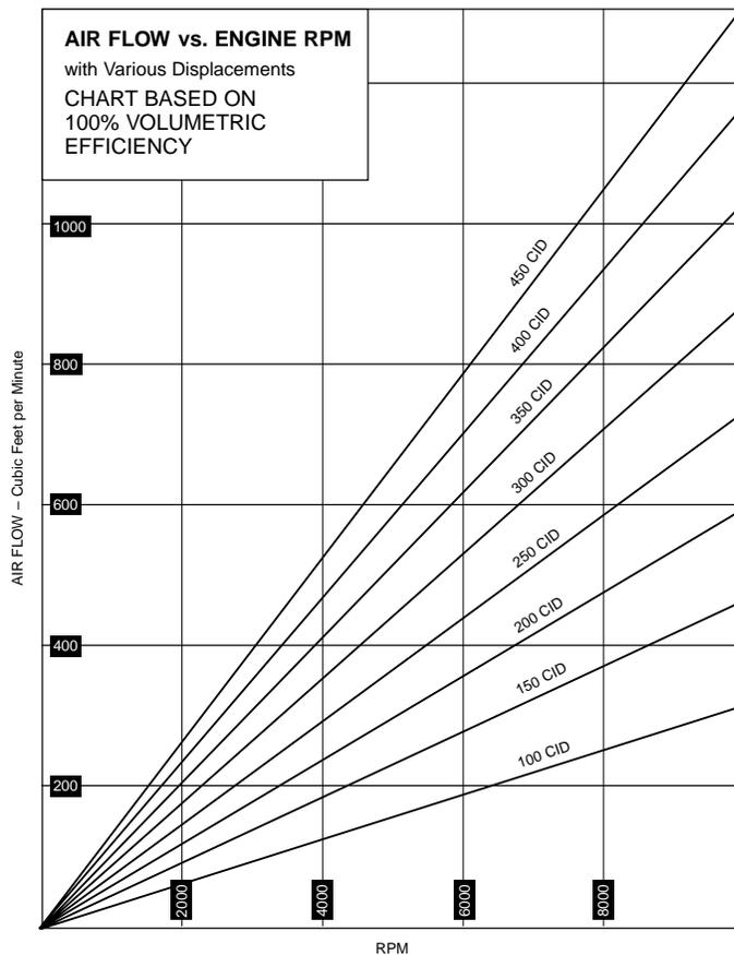
Let's take for example, a 300 C.I.D. V-8 which has a maximum RPM limit of 8000 RPM. It's been determined that this particular engine has a volumetric efficiency of 85%. According to our chart the engine's airflow requirement is 700 C.F.M. at 100% volumetric efficiency. At 85%, however, the C.F.M. requirement is 595 C.F.M. This engine would, therefore, require a 600 C.F.M. carburetor.
