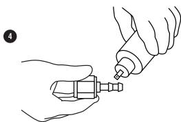
4. Lubricate the inside of the hose and the outside of the nipple. Use assembly lube or engine oil. Do not use a silicon-based lube.
