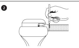
2 Place the socket in a vise and insert the end of the hose into the socket until the hose butts against the bottom of the threads provided for the cutter. Gently pull the hose back until three is a 1/16' to 1/8' gap between the end of the hose and the bottom of the threads —mark hose at bottom of socket with a felt pen so that you can detect any tendency of the hose to be pushed out as you complete the assembly.
