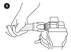
4. Holding the hose and not the socket, push the hose and the socket onto the nipple until the socket threads can be started on the cutter. Holding the hose and not the socket, start the threads and go as far as you can by hand. Depending on the size of the hose, some force may be necessary in this part of the operation.
