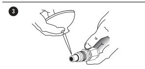
$\pmb{3}$  Lubricate the inside of the hose, the cutter threads and the socket threads with Earl's assembly lube or engine oil. Place the nipple in a vise.
