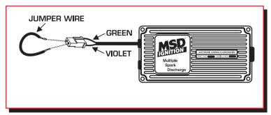
Checking for spark with the magnetic pickup as a trigger.
