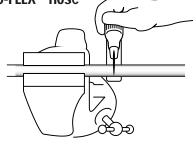
Assemble the tube-mate end onto the hose onto the hose per Auto-Fit hose and instructions.
