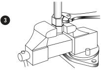
3. Using the TUBE-MATE grooving tool, groove the tubing. The tubing may also be beaded (or barbed). See Earl's new tube beading tool.
