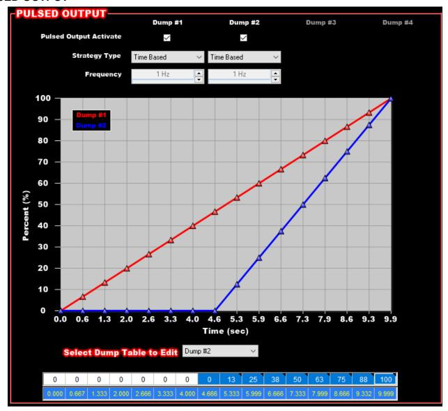
Pulsed Output and Checkbox – If enabled, the output is pulsed based on the Strategy Type of RPM or Time. The Frequency must be set. The 1x16 time/RPM axis is user editable individually for each output.
