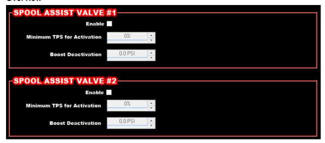
There are two Spool Assist outputs. They perform identical operations (operate only when on the transbrake). The Spool Assist outputs are intended to activate when the Race Trans Launch input (transbrake) is active and when the TPS is over the Minimum TPS for Activation. The output will turn off when the "Boost Deactivation" value is met. It will also deactivate when the Race Launch input turns off or the TPS goes below the Minimum TPS for Activation.
