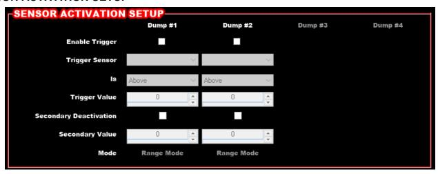
• Sensor Enable and Setup – Each output has an optional sensor trigger condition that can be used to turn the output on or off. Note that this condition does not affect the timer, just the output state (whether it is physically on or off).
