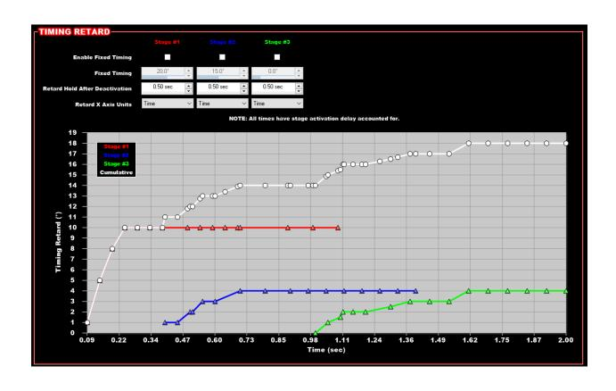
In the same manner progressive stages are shown on a summary screen. The start begins at the stages "stage activation delay", which can't be move to a value before this (modify the Stage Activation Delay).
