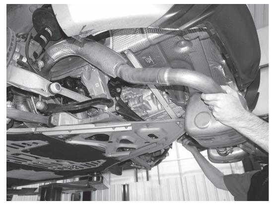
7) Lower the rear portion of the rear muffler assembly, manuvering the front portion of the rear muffler assembly away and back from the rear susension. Remove the rear muffler assembly from the car.
