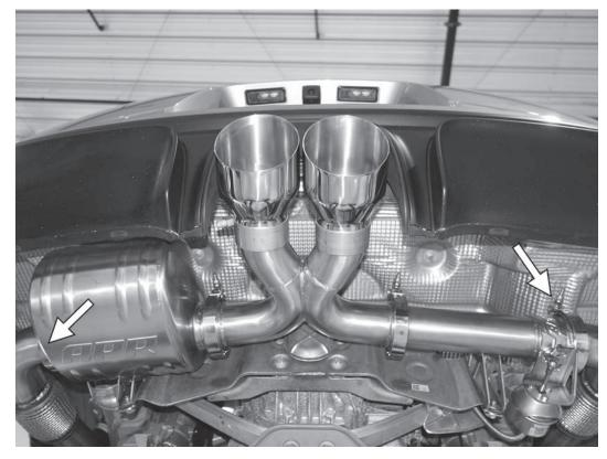
27) Adjust the APR exhaust system so the exhaust tips sit correctly in the cutout of the rear valence. You might need to rotate the exhaust on the inner or outer connections of the V-band clamps, and/or adjust the exhaust tips on the rear center section of the exhaust. Once happy with the fitiment, tighten the two outer V-band clamps first to 15Nm (11 ft-lbs).
