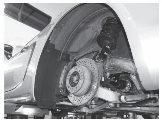
1) Securely support the vehicle on a lift or jack stands, and remove both rear wheels.
