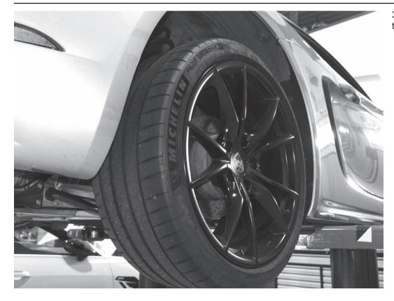
31) Reinstall the rear wheel, and torque to the correct specification.
