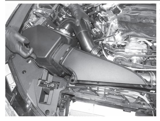
7) Lift the entire airbox assembly straight up and out of the car, with the front inlet scoop and plastic air inlet hose attached.
