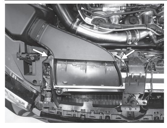
5) Remove the two T30 screws holding the front intake scoop. Lift the scoop to remove it from the car.
