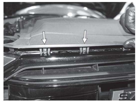
29) Reinstall the upper cover that goes between the front grille and the top of the radiator support. Ensure the tabs on front of the cover are aligned with the slots on the top of the grille before pushing the front of the cover down and in place. Not aligning these tabs can bend and distort them.
