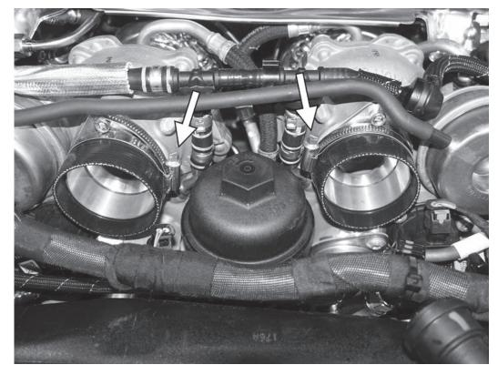
17) Install the two APR silicone couplers with two of the supplied hose clamps. Orient the clamps for easy access when tightening.
