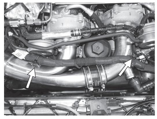
9) Unclip the two attachment points for the factory wiring harness that runs along the top of the stock metal inlet tube.
