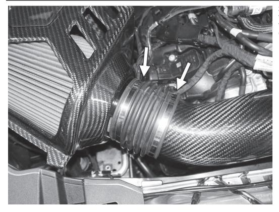
25) Making sure the coupler is centered, adjust the two clamps and then tighten both of them to 3.5Nm (31 in-lbs).
