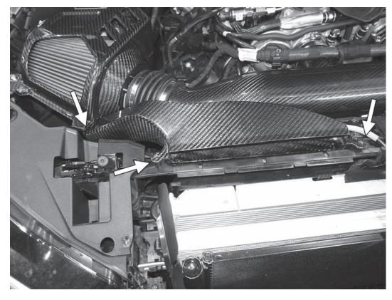
27) Place the APR intake scoop onto the APR airbox. The screw holes on the inlet side of the scoop should align with the screw holes for the factory air ducting.
