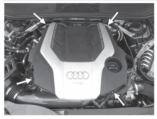
33) Reinstall the engine cover by pressing the cover down onto the four mounting posts on the engine.
