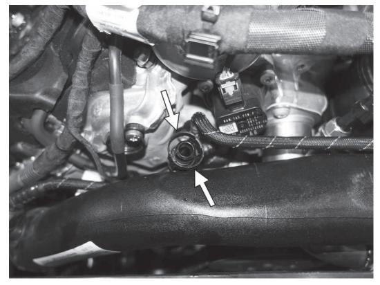
13) The PCV connection can be easily removed by squeezing in on the two wider sides of the connection.
