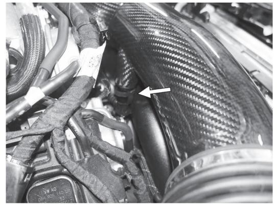
19) Place the APR carbon inlet tube close to its resting spot on the engine. Reconnect the PCV connection to the bottom of the APR inlet tube by pushing it into place.
