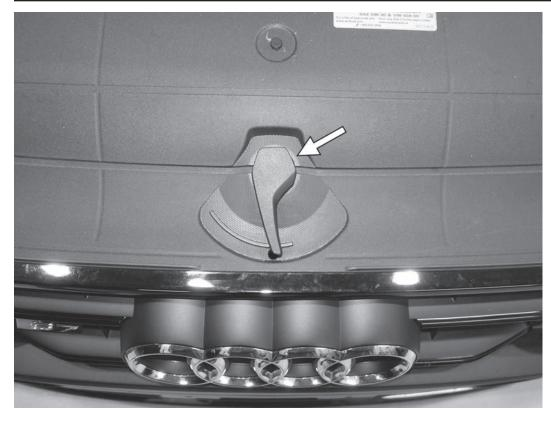
31) Reinstall the hood latch to the mounting post in the center of the upper cover. The post and latch are keyed, so it will only go on in one direction. Simply push down on the latch until it clicks to lock it in place.
