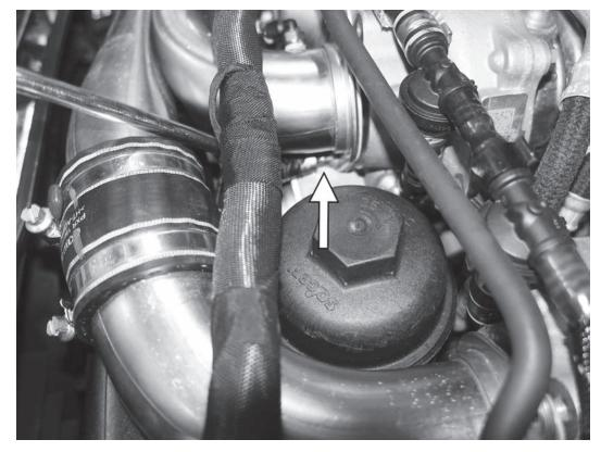
11) On the lower two T30 screws that hold the inlet pipe to the turbo, use a magnet to hold the screw as you remove the screws. This will prevent the screws from falling down in the engine, as they will be reused.
