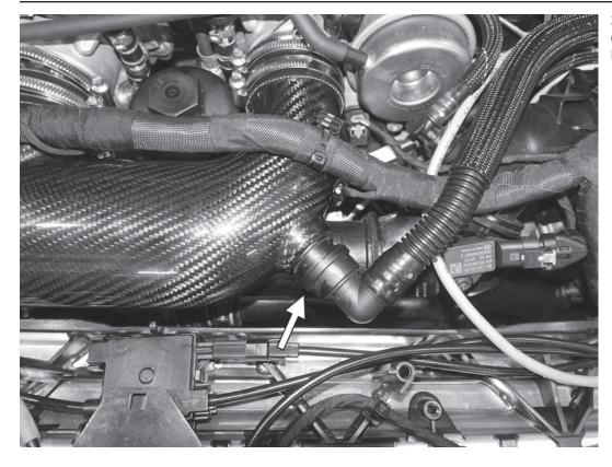
21) Reconnect the PCV connection onto the front of the APR inlet tube by simply pushing the fitting in place.
