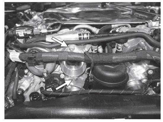
15) Install the billet adapter with the captured screw and gasket on the front of the right turbo. Install the screw into the lower hole on the turbo inlet and start threading the screw. Install the upper T30 screw through the adapter and gasket and thread into the upper hole on the front of the turbo. Torque both the upper and lower T30 screws to 9Nm (80 in-lbs).
