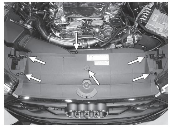
3) Remove the five T30 screws holding the cover between the front grille and the radiator support. Also remove the one push pin style connector in the middle of the cover. To remove this pin connector, carefully pry the raised center part of the pin up, and then remove the entire pin assembly up and out of the cover.
